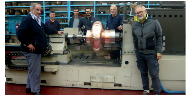
Two Copper 400 MHz seamless Prototype realized
