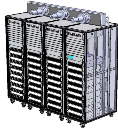
INFN prototype of solid state amplifier (200 kW cw, 175 MHz), under construction in the national industry. To be delivered May 2022
