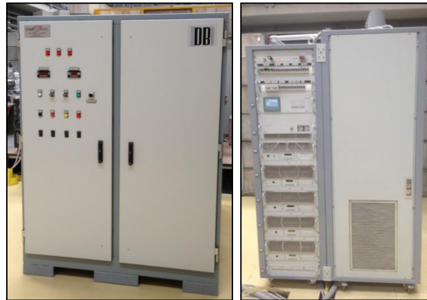
Two stages tetrode based amplifier (200 kW cw, 175 MHz), installed in 2013 used for high power tests of IFMIF RFQ segment, built in national industry
