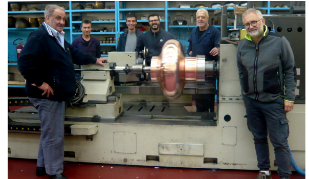
First 400 MHz seamless elliptical cavity prototype
