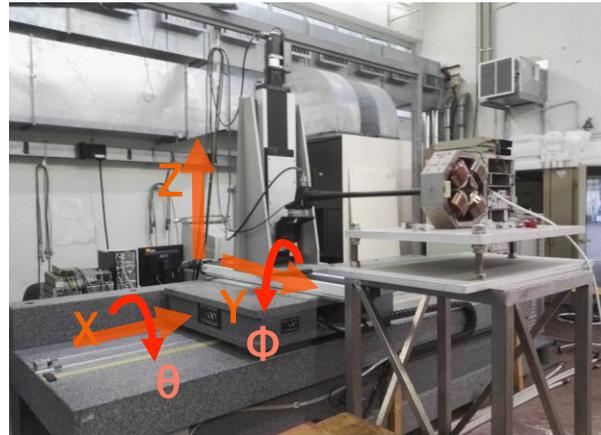
5-axes digital Movement device equipped with
