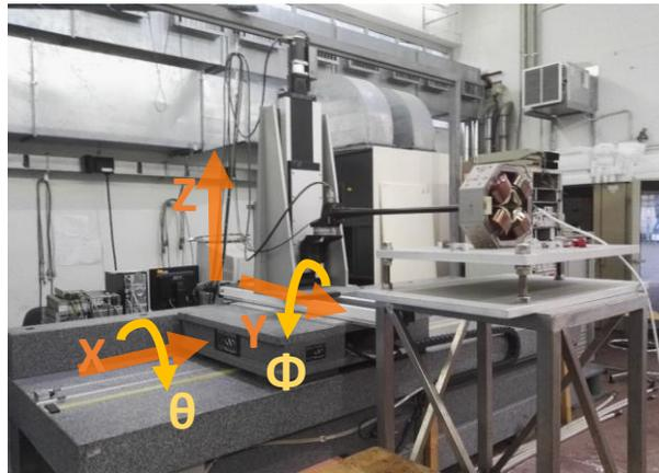
5-axes digital Movement device equipped with Hall Probe
