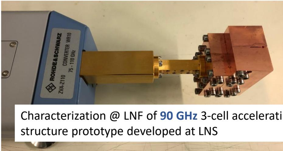
Characterization @ LNF of **90 GHz** 3-cell accelerating structure prototype developed at LNS
