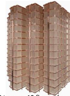
19 towers 13 floors 4 crystals = 988 bolometric crystals
