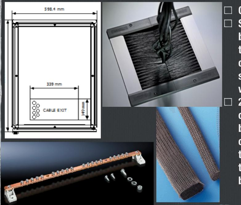
**Cable entries : top of the cabinet** Sealing of the cable openings will be performed with the use of air tight brush type sealants in most of the racks and with EMC sponge type sealants in the cases where EMC should be considered 2 earthing bars, the one connected to the equipotential bonding bar (PB) and the other one connected to the EMC grid through the gallery floor pads or the wall mounted grounding bus bar
