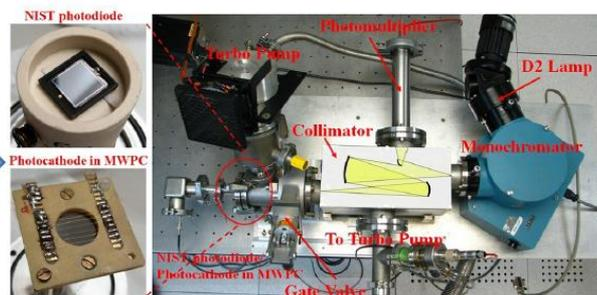
**Apparatus for QE measurements**
