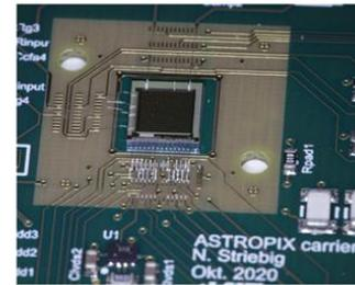
(b) Picture of the AstroPix V1 detector on a carrier board.
