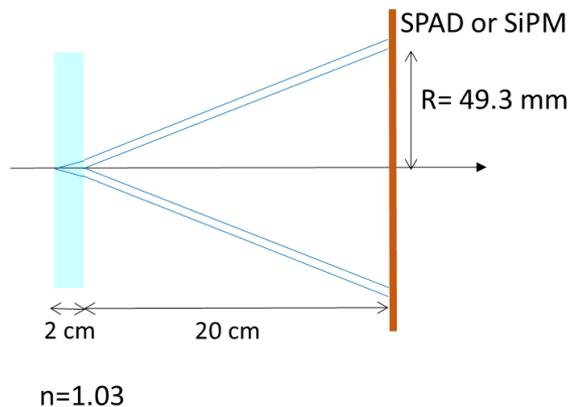
Double layer aerogel -> focusing, reduced geometric aberration
