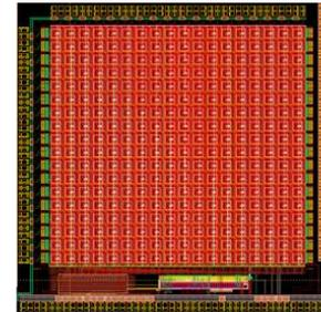
(a) Top level view of the AstroPix V1 sensor matrix. The matrix is 18 by 18 pixels, each pixel  $200 \mu\text{m}^2$ , with digital readout for each row and column.
