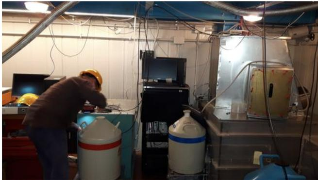
Connection of the Front-End electronic to the BEGe's Canberra preamplifier (Mod. 2002C), behind the liquid N<sub>2</sub> dewar
