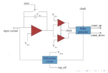
The front-end circuit has been successfully designed by Torino group in different technologies (not yet in 28 nm)
