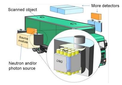
The system detects fission gamma rays and fast neutrons emitted spontaneously or by stimulation from nuclear materials
