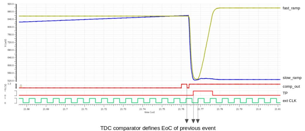
Test-pulse arrives before next clock cycle (internal clock is shifted w.r.t. external CLK)
