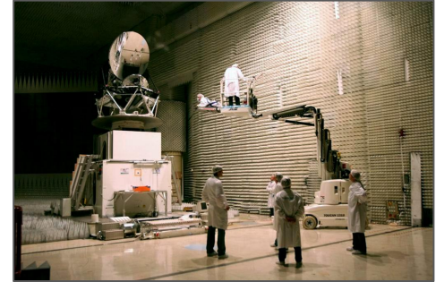
CATR setup at Thales Alenia Space
