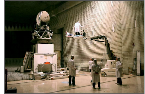
CATR setup at Thales Alenia Space
