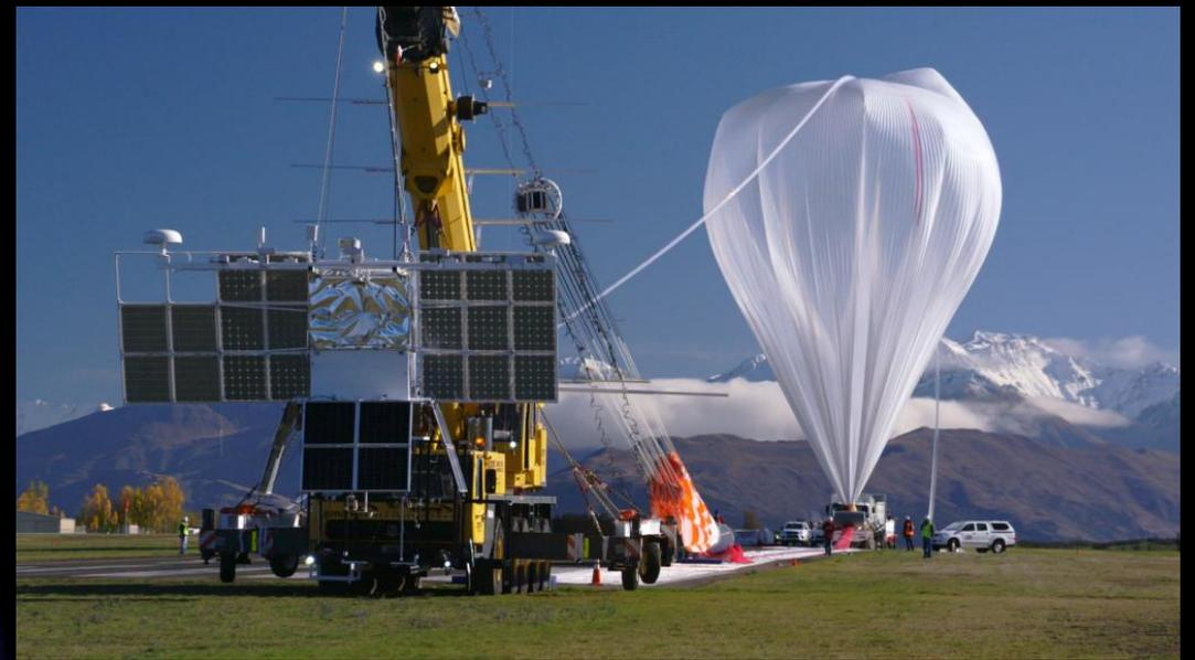
Great progress with super-pressure balloons: COSI payload flown by CSBF in may 2016 for 47 days at altitudes between 33 km and 21 km, with a with a  $0.5\text{Mm}^3$  SPB
