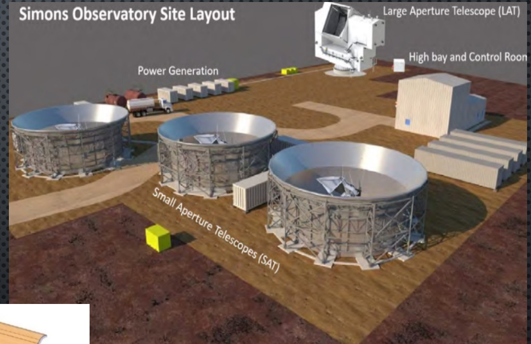
SO Small Aperture Telescopes inside their large ground screens
