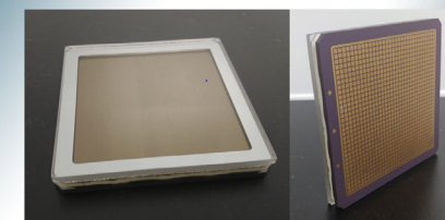
10 cm x 10 cm MCP-PMT 1024 readout pads (2.5 mm x 2.5 mm)
