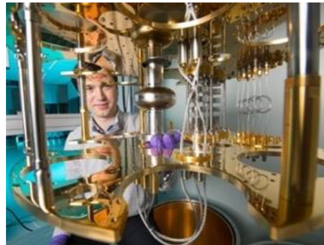
Dilution Fridge at FermilabAPS-TD Quantum Lab (QCL)
