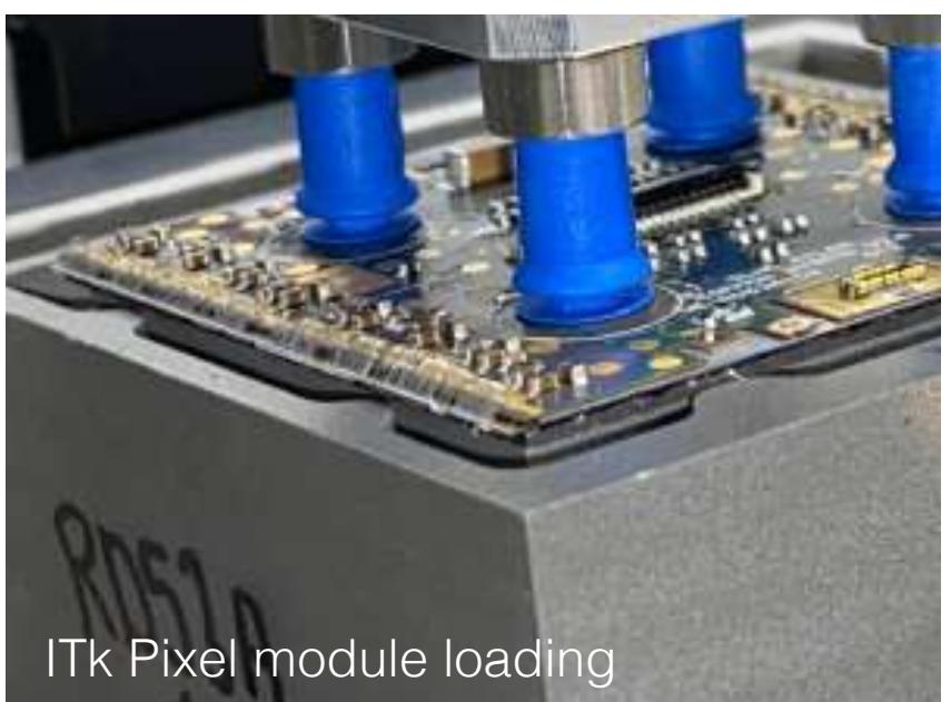
ITk Pixel module loading
