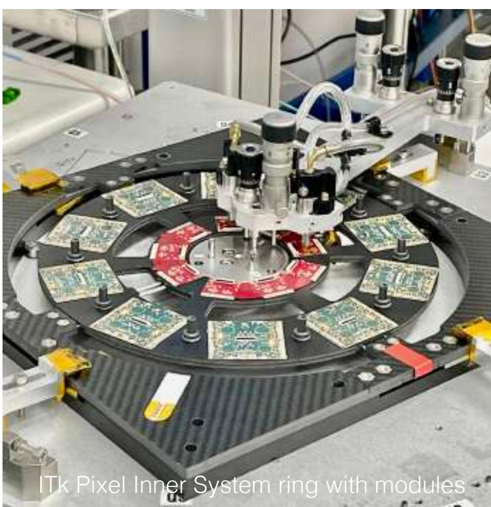
ITk Pixel Inner System ring with modules
