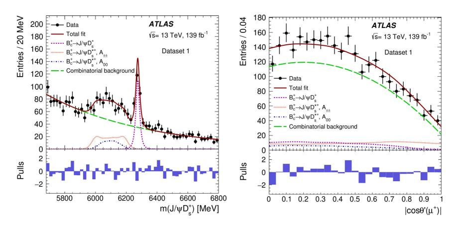
Left: fit to inv. mass m(J/ $\psi$ D<sub>s</sub><sup>+</sup>). Right: fit to |cos  $\theta$ '( $\mu$ <sup>+</sup>)|, where  $\theta$ '( $\mu$ <sup>+</sup>) is the helicity angle between  $\mu$ <sup>+</sup> and D<sub>s</sub><sup>+</sup> momenta, in J/ $\psi$  rest frame.
