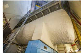
Cryostat covered in insulating foam
