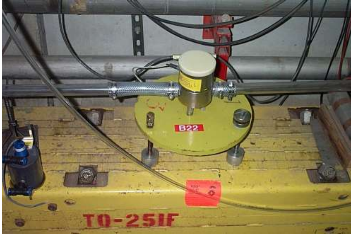
Fig.35. HLS probe on Tevatron accelerator focusing magnet.
