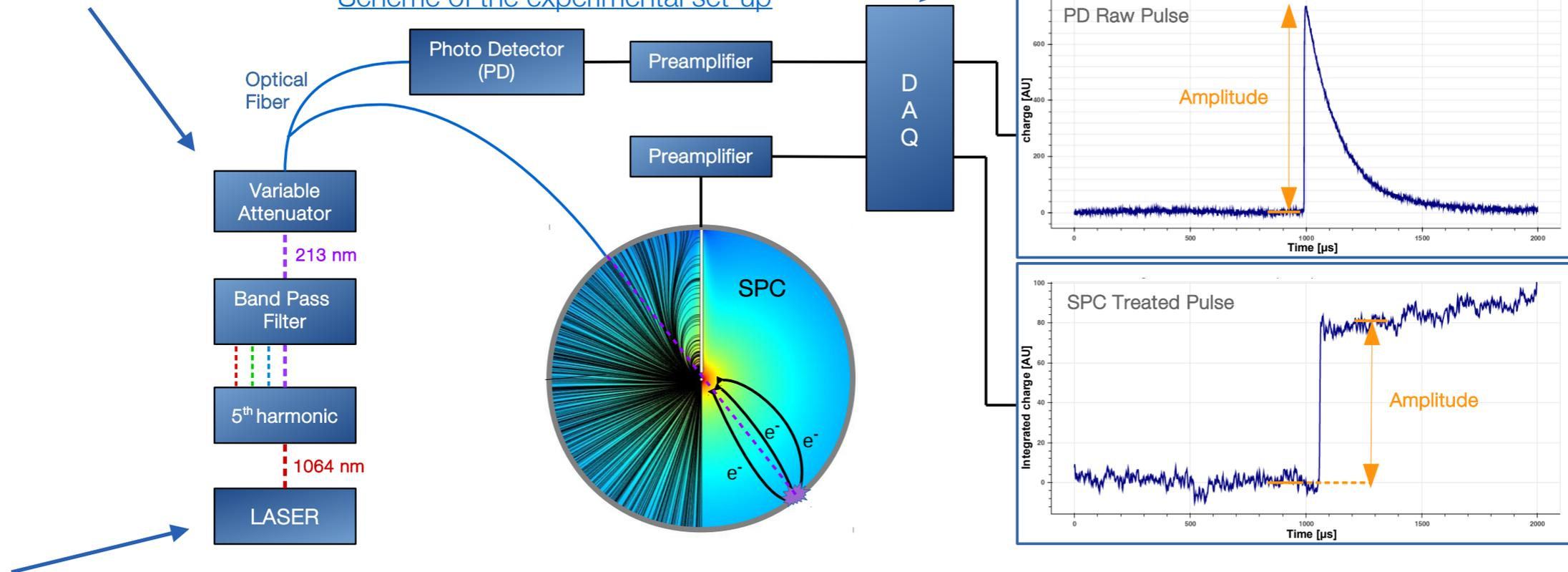
A powerful UV laser capable of extracting 100s of electrons
