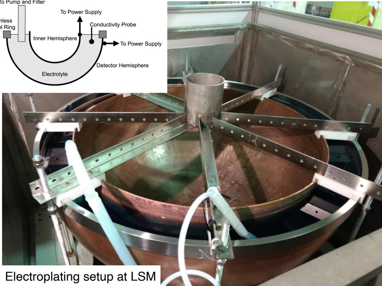
Electroplating setup at LSM
