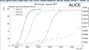
The main standard gas mixture component, the  $C_2H_2F_4$ , is now substituted by a proper mixture of  $CO_2/C_3H_2F_4$  (HFO1234ze). The HFO is used as quencher, while the  $CO_2$  is used to decrease the operating voltage in order to work with lower current.
