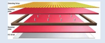
In High Energy Physics the RPC are widely used for triggering thanks to their excellent time resolution (<1 ns) and velocity. The low cost per unit area make them suitable to be used in large area experiments, like those operating at the Large Hadron Collider. At LHC they operate in avalanche mode by means of the standard gas mixture
