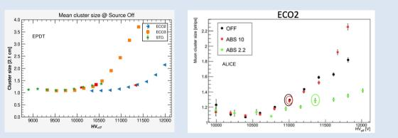
The average cluster size is comparable at the working point for the three gas mixtures, both with source off and under irradiation
