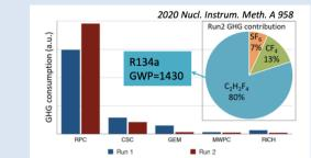
The F-gases, like  $C_2H_2F_4$  and  $SF_6$ , are now considered to be non-eco-friendly for their high Global Warming Potential (GWP), which represents the measurement of the greenhouse impact of a
