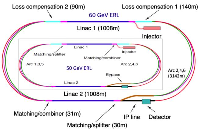
An intense electron beam (20mA current) is accelerated in three passes through two 1km linacs in an energy recovery linac racetrack configuration, which is positioned tangentially to the LHC (at IP2, or L for FCC).
