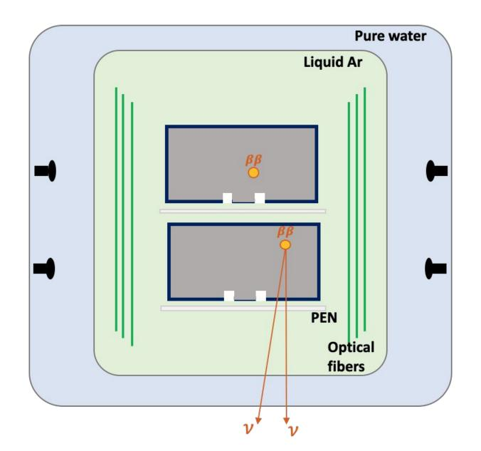
ββ decay signal: single energy deposition in a 1 mm<sup>3</sup> volume
