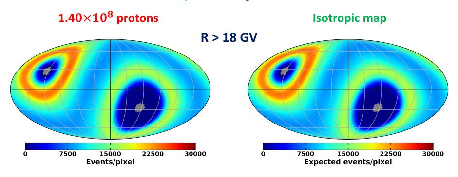
For the anisotropy analysis, selected events are grouped in **9 cumulative rigidity ranges**:  $R_{min} > 18, 30, 45, 80, 150, 200, 300, 500$  and 1000 GV
