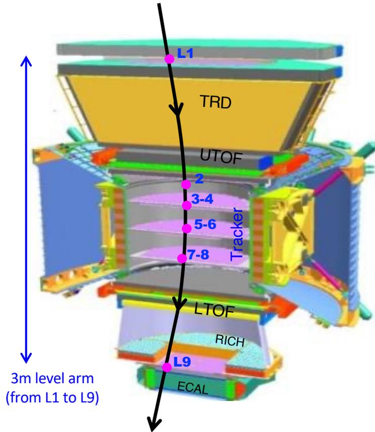
**Particle Rigidity** (momentum/charge) is measured combining Tracker (9 Layers) + Magnet
