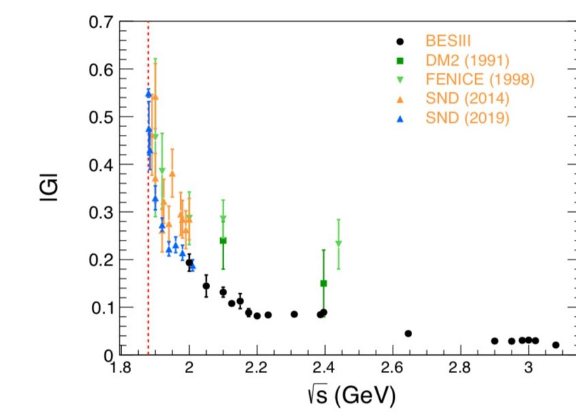
$$\sigma_{Born} = \frac{N_{data}}{\epsilon_{nn}^{MC} \times \mathcal{C}_{dm} \times \mathcal{C}_{trg} \times (1 + \delta) \times \mathcal{L}_{Int}} \quad |G_{eff}| = \left( \frac{3q^2}{4\pi\alpha^2\beta(1 + \frac{2m_n^2}{q^2})} \right)^{\frac{1}{2}} \sqrt{\sigma_{Born}}$$
