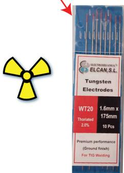
Thoriated welding electrodes (2% <sup>232</sup>Th) were used a radioactive source; they can be a good choice for a system in a school or for a portable physics lab. Furthermore, <sup>232</sup>Th has lots of clearly identifiable peaks: it can be used as a calibration source.
