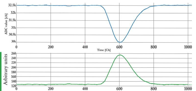
Signal shaped by a RC4 software filter. After subtracting the baseline, the time information and the pulse height are computed.
