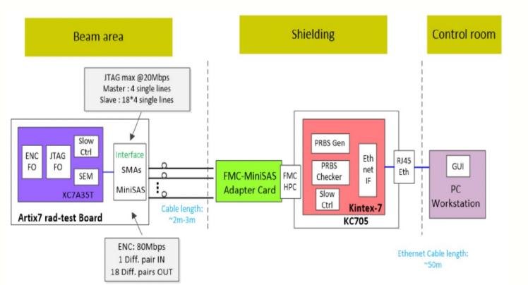
The beam area is the DUT (Artix-7) with a test firmware connected through FMC-miniSAS cables to the DAQ Firmware (KC705) shielded from the beam.
