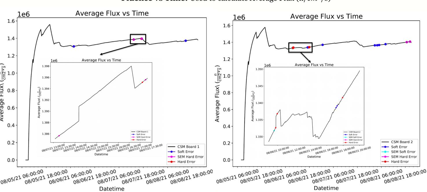
Average Flux vs. Time: CSM 1 with 5 SEU Errors -2 Soft Errors, 1 Hard Errors, and 2 SEM Hard Errors (categorized in the end as Hard Errors)
