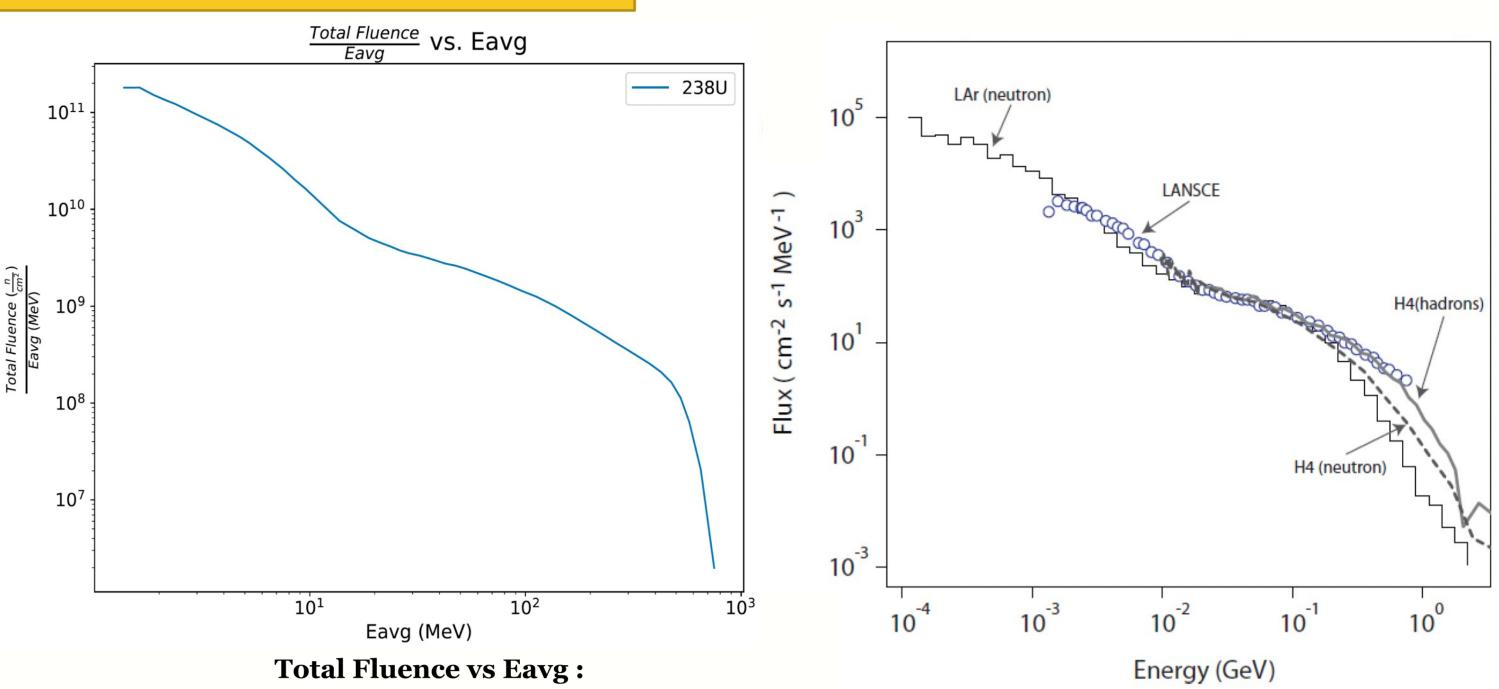
Energy spectrum at LANSCE during Beam run **ATLAS LAr Detector Sample Energy Spectrum Plot**
