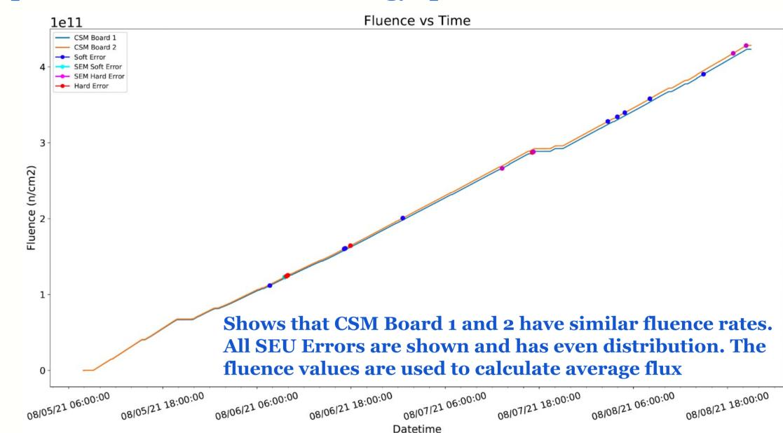
**Fluence vs Time:** Used to calculate Average Flux  $(n/cm^2/s)$
