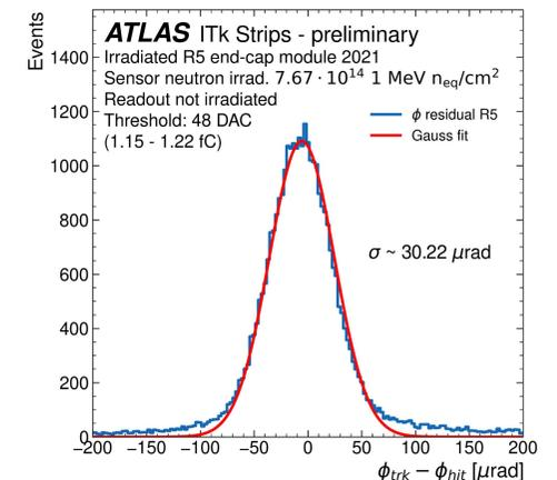
Angular resolution for the R5 module displayed above.
