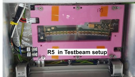
The first *end-cap* split-module (R5 type) was tested in December 2021. Sensors were irradiated with neutrons at JSI Ljubljana, to 7.67 · 10<sup>14</sup> 1-MeV n<sub>eq</sub>/cm<sup>2</sup>. Front-end electronics were not irradiated.
