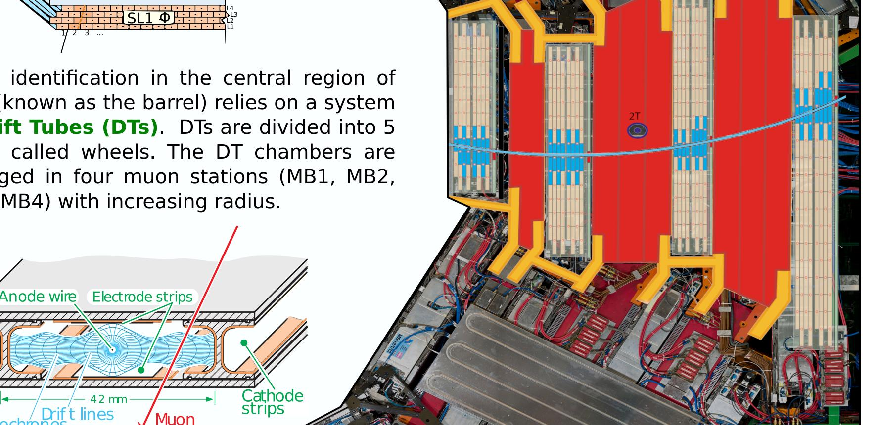
DT systems consist of gaseous detectors capable to detect the ionization signals caused by particles traveling through them. When those signals are received by the read-out electronics, they are digitized into "**hits**".
