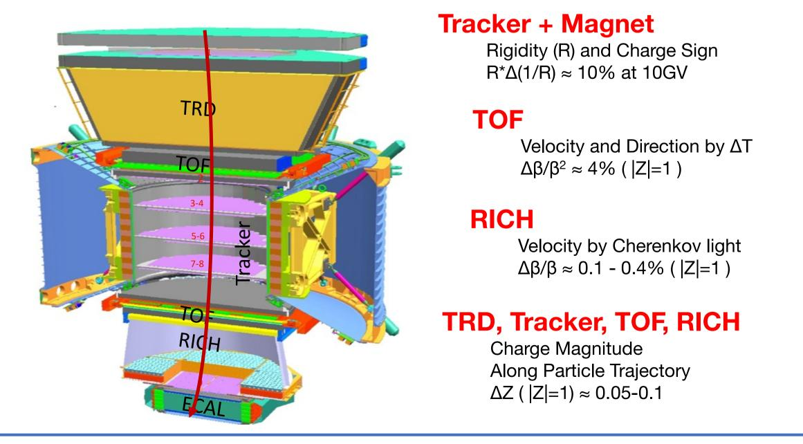
One of the unique properties of AMS in space is that events can be classified with different subdetectors. For example, secondary particles produced by interactions inside TRD can be identify with the velocity differences in TRD and TOF and the mass reconstructed with TOF and Tracker.
