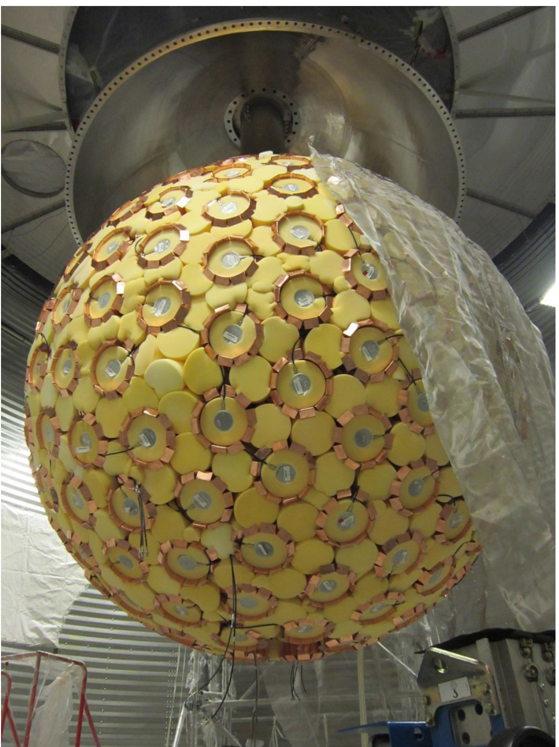
Figure 1. Left: cross-sectional representation of DEAP-3600. Right, top: the stainless stell shell, containing the acrylic vessel and the instrumentation, inserted into the cylindrical water tank. Right, bottom: acrylic vessel after the mounting of the PMTs and the polyethylene inserts.
