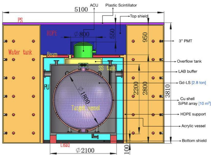
Fig. 1: Schematic view of TAO detector
