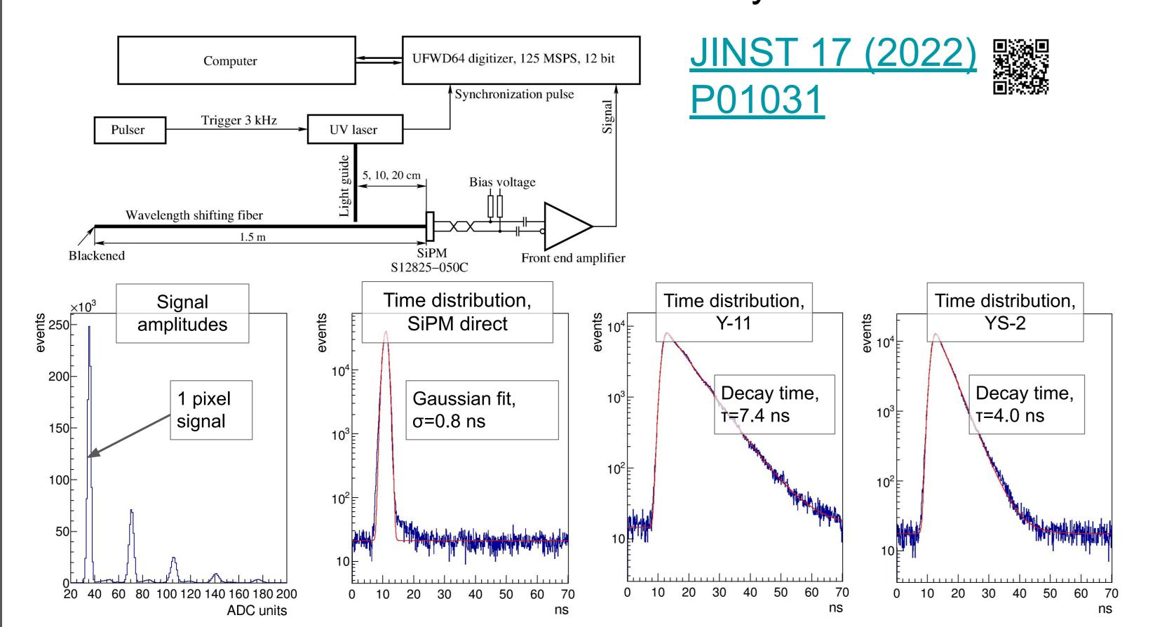
Single pixel events only are used ⇒ no time walk, etc. In case of Gaussian hardware resolution with width σ and exponential emission decay with time T event distribution is given by:
