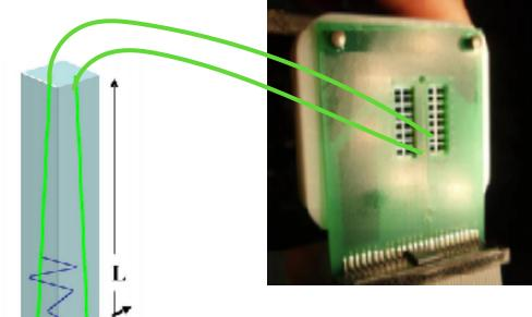
Wavelength shifting fibres read out by a single pixel on Avalanche Photodiode
