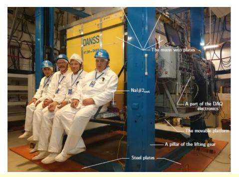
DANSS is installed on a movable platform under 3.1 GW WWER-1000 reactor (Core:h=3.7m, ∅=3.1m) at Kalinin NPP. ~50 mwe shielding => µ flux reduction ~6! No cosmic neutrons!
