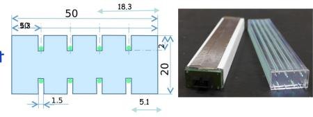
WLS fiber positions were optimized for better uniformity of response New fast (4ns decay time) YS2 fiber will be used
