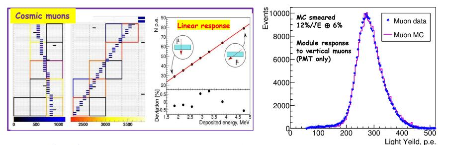
Several calibration sources are used to check the detector response
