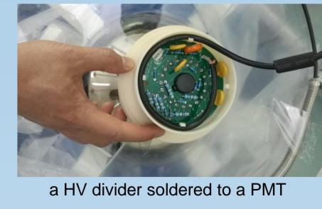
Circuit design for dynode-PMT
