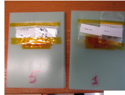
LGAD and AC-LGAD test samples under irradiation tests at LANL.
