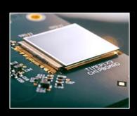
TIMEPIX Array a digital Camera for real time radiation monitoring
