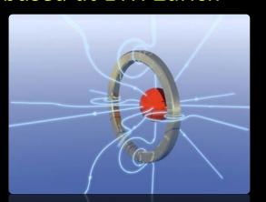
Signal for a monopole is a continuing current in the SQUID after the monopole has passed through
