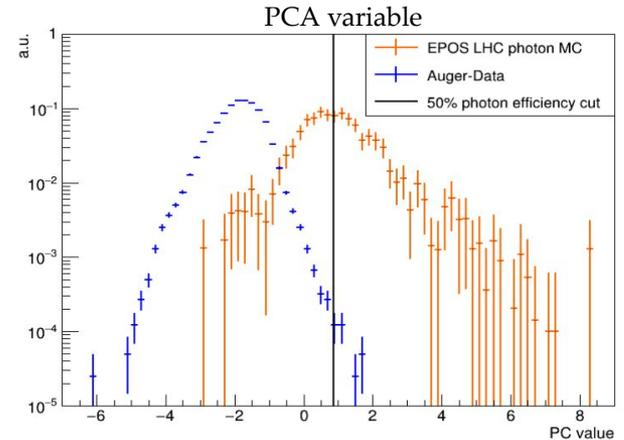
Cut set to have a 50% efficiency on the photon signal
