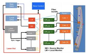
Calibration of the 1296 crystals for Short Term  $\mathcal{O}(1 \text{ ns})$ , Measurement Window  $\mathcal{O}(1 \text{ ms})$  and Long Term  $\mathcal{O}(1 \text{ day})$
