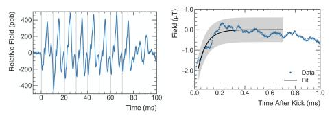
Transient B-field from the quadrupole plates vibration during the pulse. The grey bands represent the measurement window. Transient B-field  $\sim$  200 G from the kicker Eddy Currents. Measured with a *Faraday Effect* magnetometer.
