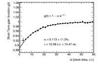
Gain function to correct for the SiPM bias voltage recovery time due to the large number of particles hitting the calorimeters. Laser pulses (known energy) are sent in the calorimeters at different times to measure the response function.
