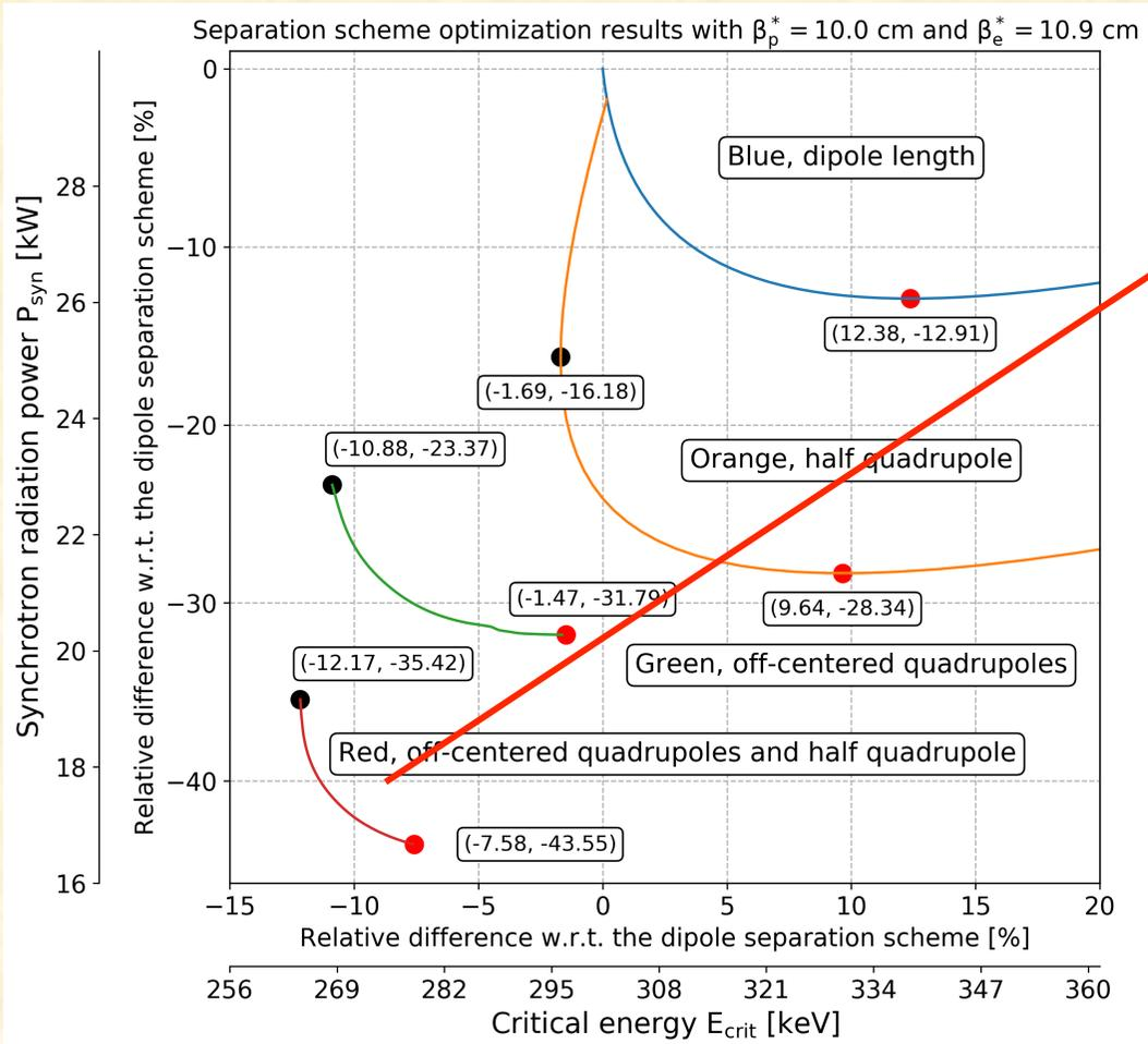
*combine a detector integrated dipole field with an early focusing scheme, off-centre quadrupoles ( $1/\rho = const$ ) and very compact proton quadrupole design*
