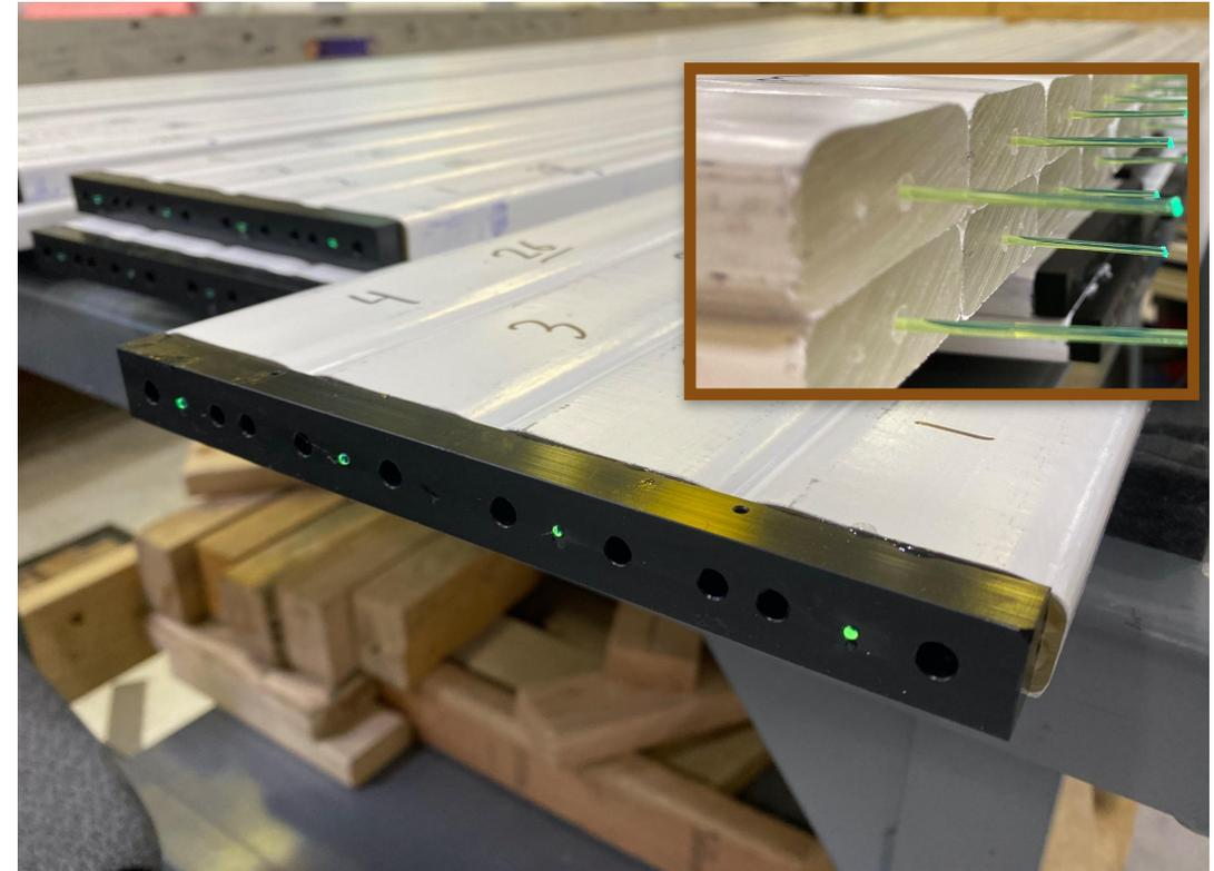
**Hadronic calorimeter scintillator bars layer**
