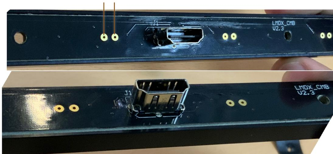
Backside of control board, showing HDMI port & SiPM probe points
