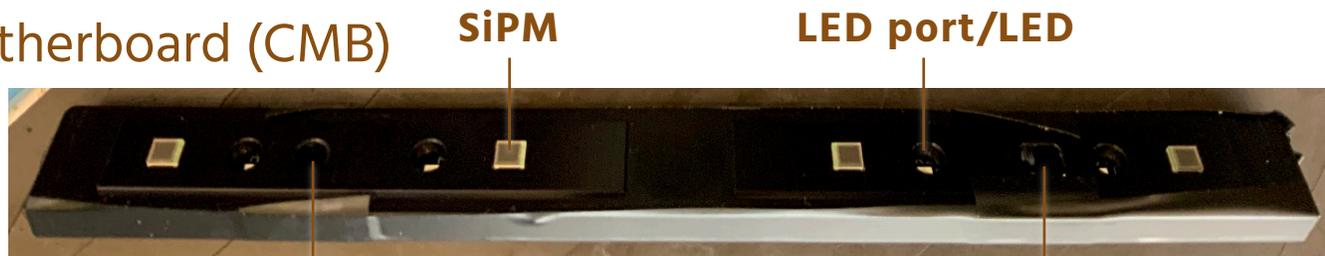
**Screw hole (circular)** Front panel with SiPMs visible
