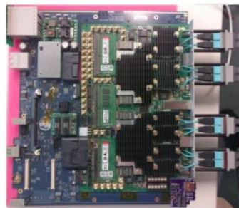
L0 muon trigger board prototype
