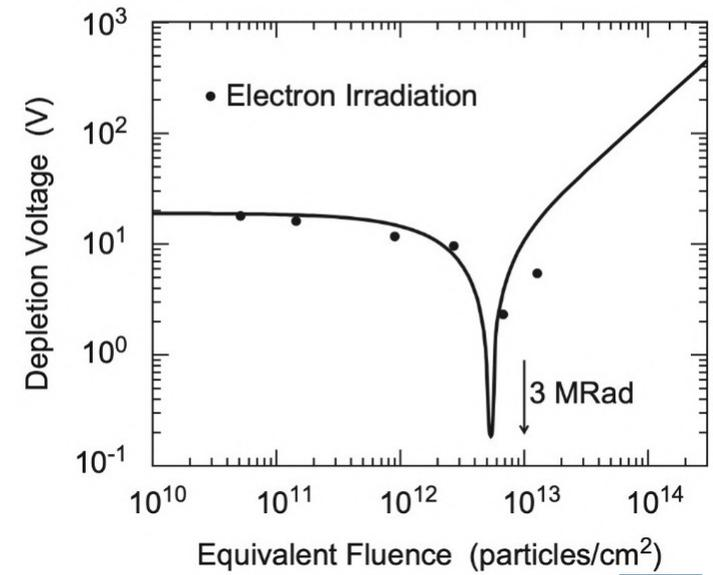
No change in full depletion voltage observed with time so far, consistent with low integrated neutron fluence(  $\sim 1.6 \times 10^{11}$  neq/cm<sup>2</sup>)
