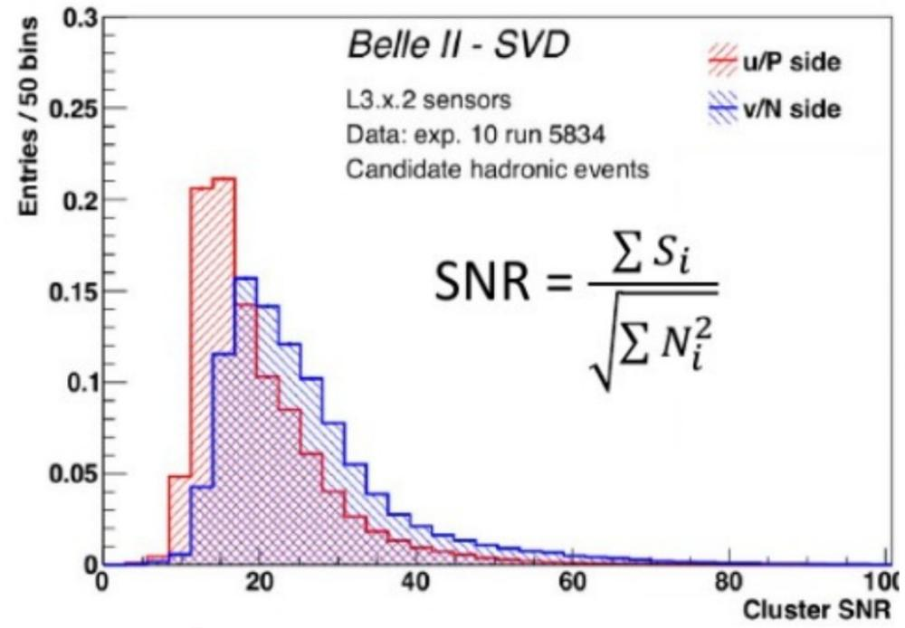
u/P side: larger noise due to longer strip length (larger inter-strip capacitance)
