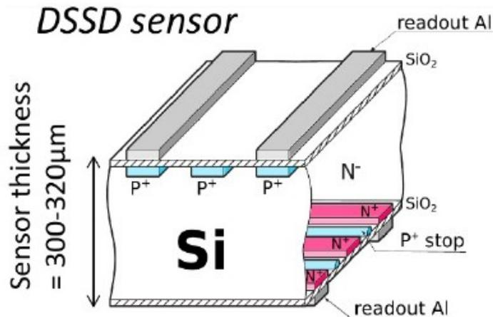
AC-coupled strips on N-type substrate
