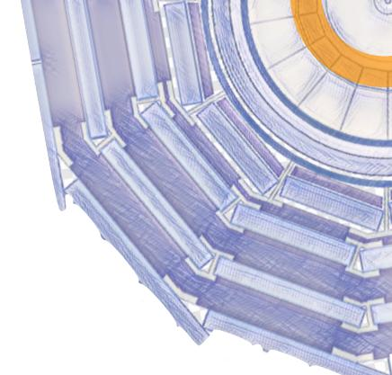
A homogeneous, hermetic, high granularity PbWO<sub>4</sub> crystal calorimeter...
