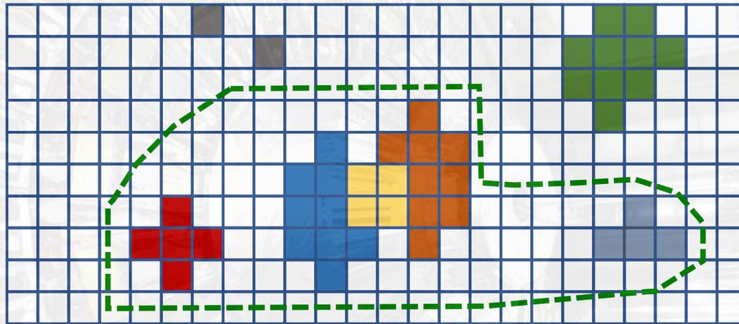
Refined superclusters use the information from the tracker, to be able to link bremsstrahlung emissions to missed ECAL deposits
