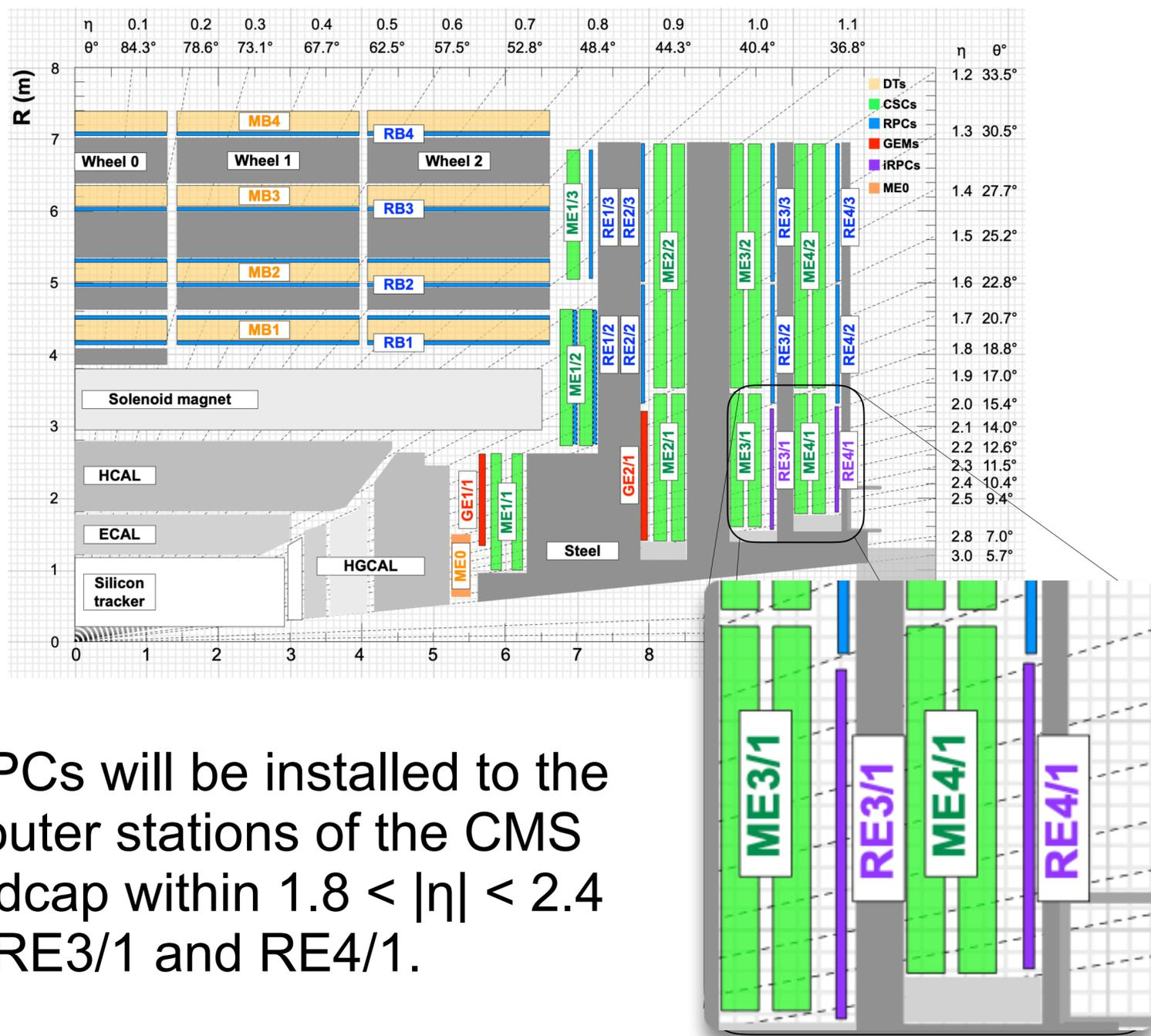
iRPCs will be installed to the 2 outer stations of the CMS endcap within  $1.8 < |\eta| < 2.4$  in RE3/1 and RE4/1.
