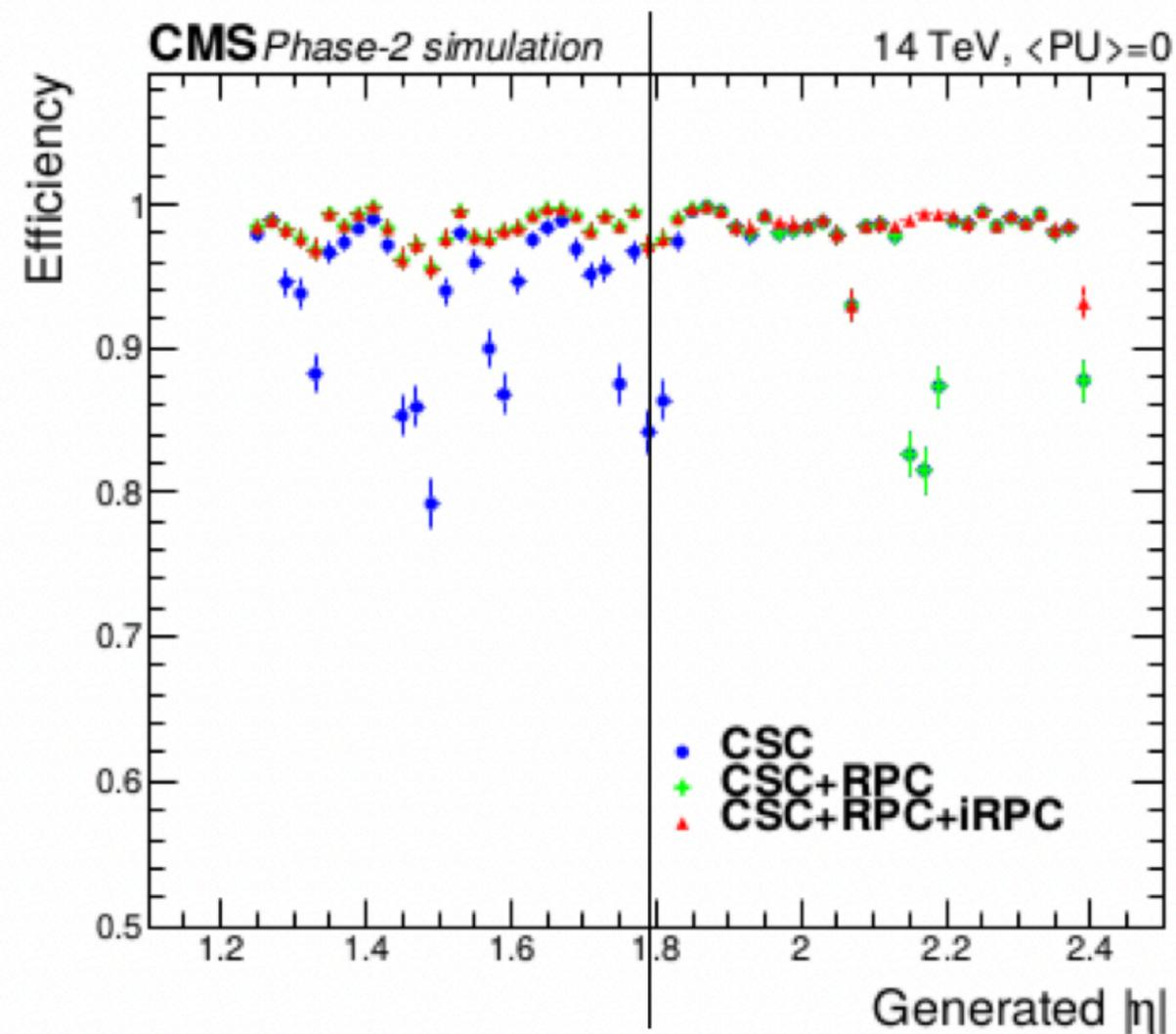
Efficiency  $> 90\%$  everywhere if iRPC hits in the endcap muon track finder trigger algorithm RE4/1.
