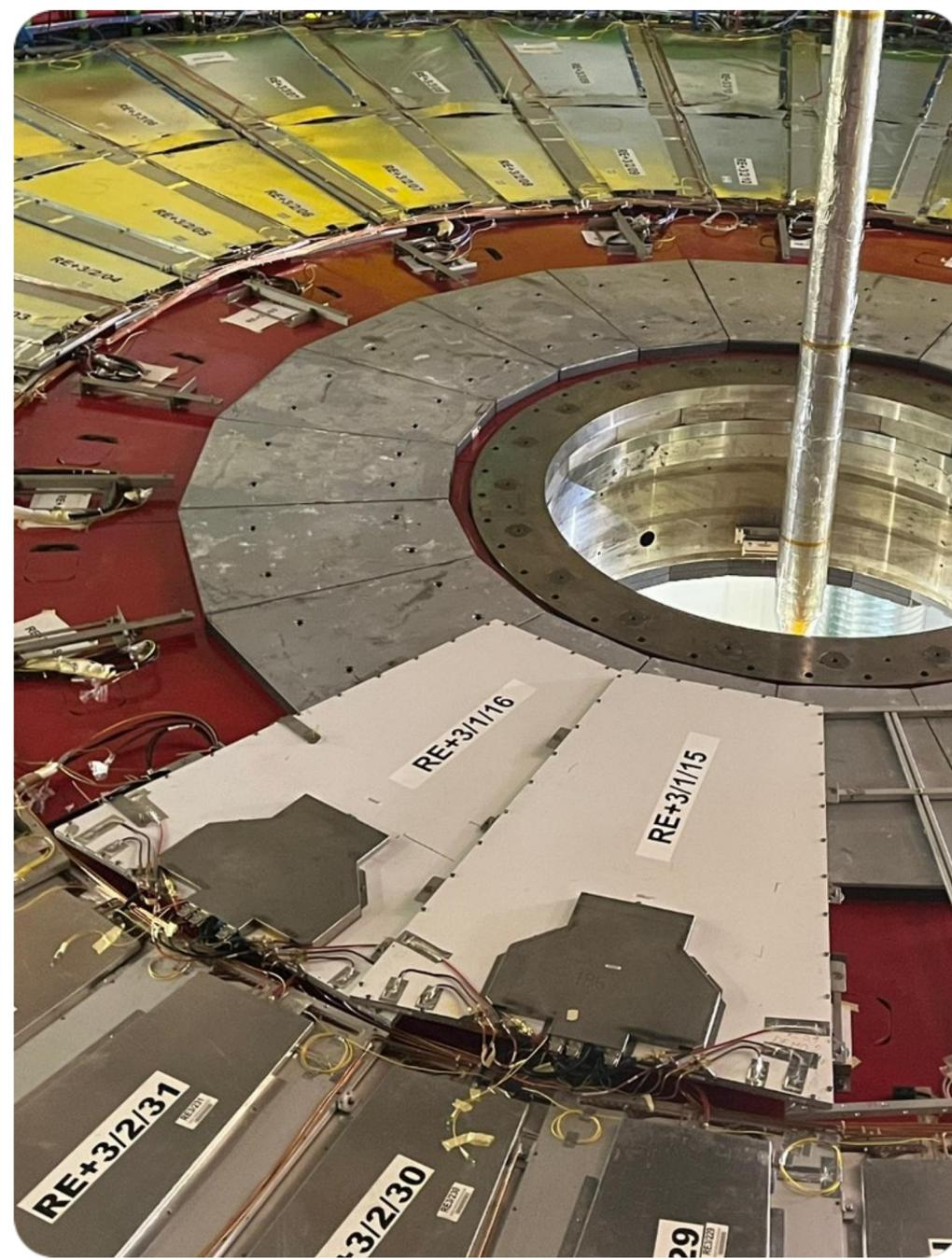
Four demonstrator chambers have just been installed in CMS cavern at the end of LS2. The picture on the left to right exhibit the final position of the demonstration chambers RE+4/1/15,16 and RE+3/1/15,16 respectively.
