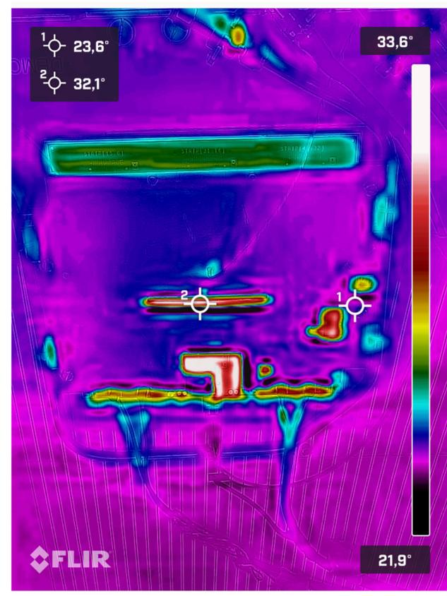
With cooling plate, Measurement with sensor: fpga 2: ~30C
