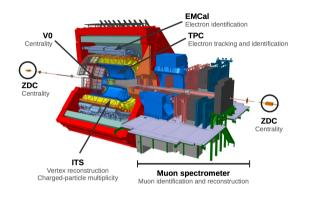
pp: Electrons reconstructed in the central barrel  $(|\eta|<0.6).$  p–Pb and Pb–Pb: Muons reconstructed in the forward spectrometer  $(-4<\eta<-2.5).$  Probing of the low ( $\sim 10^{-4}$  to  $\sim 10^{-3}$ ) and high ( $\sim 10^{-1}$  to almost unity) Bjorken-x regions.
